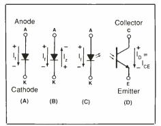
Fig. 4. Symbols and polarities: (A) rectifier diode; (B) zener diode; (C) light-emitting diode; (D) photo-diode.
