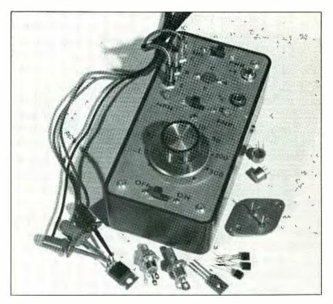
power (milliwatt) transistors to the tester. Jacks J3, J4 and J5 parallel the connections to SO1 and provide the means for connecting medium-power and high-power transistors to the tester.
