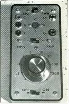
Fig. 3. Suggested front-panel layout, with appropriate panel labeling.
