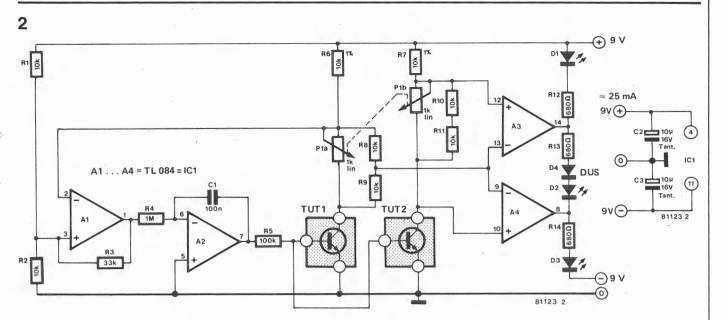
Figure 2. The final version of the circuit diagram. It is built around a set of four opamps. Two (A1 and A2) constitute the triangular wave gen or and the other two act as comparators.
