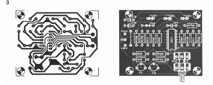
The component overlay and track pattern of the tester printed circuit board. Reliable sockets should be used for the two TUTs.
