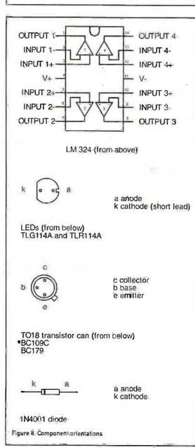
The correct orientation of the transistors, diodes and LEDs, and electrolytic capacitors needs to be observed. The polarity of an electrolytic capacitor is marked on its cover; figure 8 gives details of the physical configuration of the other components.
