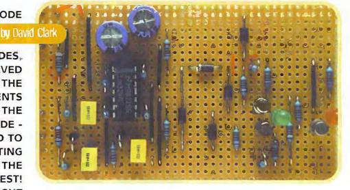
The oscillator generates a square wave at approximately 2 kHz to provide the test signal that is applied to the diode.
