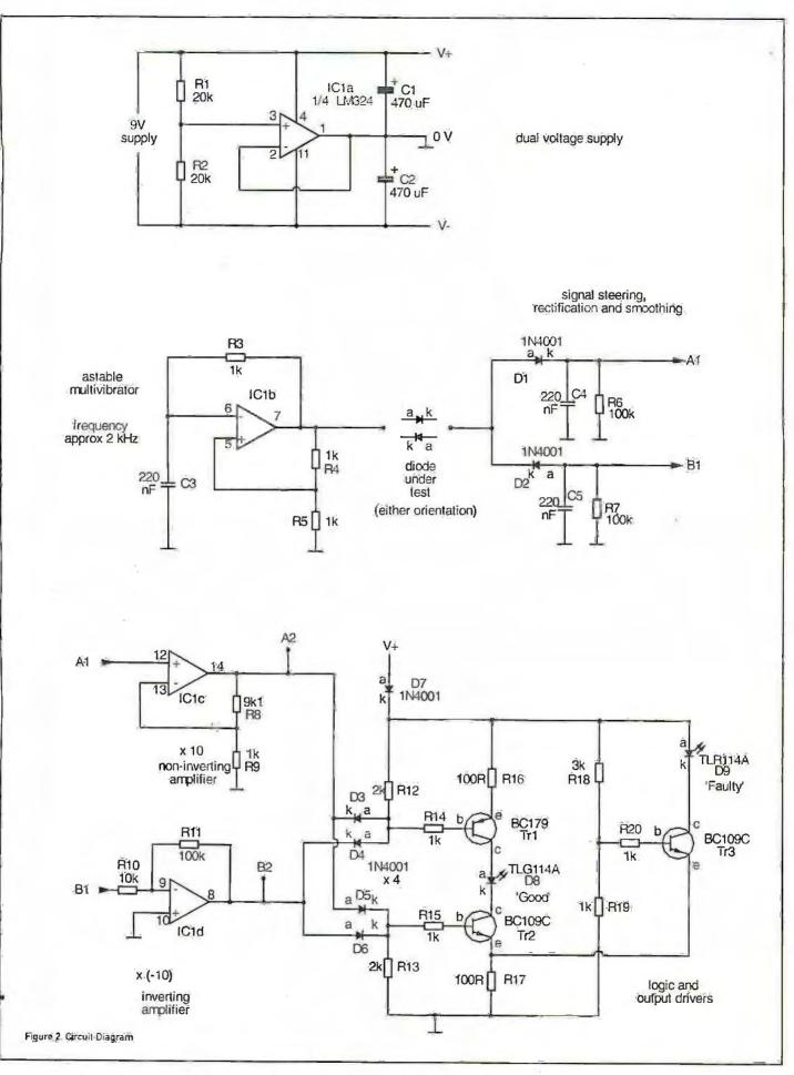
of a two-resistor voltage divider between the positive and negative terminals of the battery provides a zero volt reference point and an op-amp voltage follower maintains this. reference voltage even under varying supply current demands on both supply rails. The capacitors provide smoothing to prevent any spikes or dips appearing on the supply voltage
