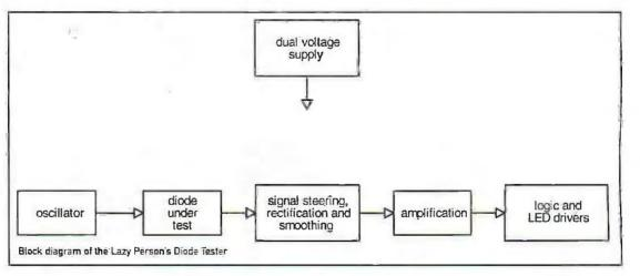
between a faulty and an OK diode.
