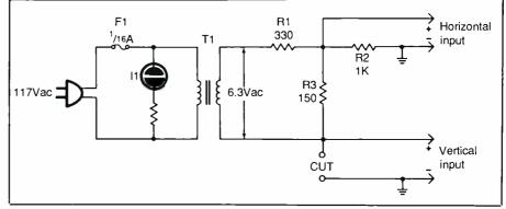
Fig. 1. Overall schematic diagram of In-Circuit Component Tester.
