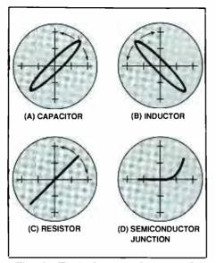
Fig. 2. Typical scope displays obtained for the most common circuit components. Traces shown are for good components. Departures from these indicate that the component being tested is defective.
