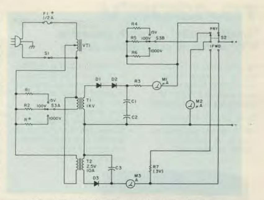
Fig. 1. The diode analyzer schematic diagram.
