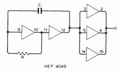
Fig. 4. Five of the six inverters in the HEF 4049 i.c. used to generate square waves.
