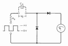
Fig. 1. Diode pump principle
