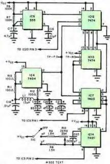
Fig. 3. Oscillator, sync., and reset circuits.
