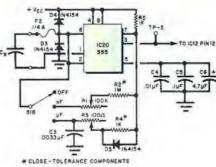
Fig. 2. Input stage has free-running 555 timer.
