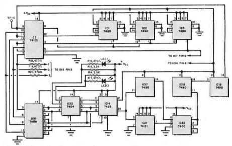
Fig. 5. Schematic of meter's autorange circuit.
