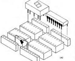
Fig. 9. A trough is provided for the current-limiting resistors as shown in (A). Diagram at (B) shows how numbering the holes allows quick resistor placement.
