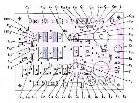
Fig. 8. Component placement guide. Numbered circles are feedthroughs.
