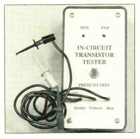
LEDs alternately flash or do not flash at all during a test, the transistor is bad.
