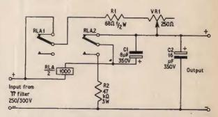
prototype a 1,000 $\Omega$  G.P.O. type relay with two sets of change-over contacts was used which closed at 5mA and with the given resistance values gave a range of cut-out currents from 20mA to 75mA. Other relays, however, of the same resistance and design may not close at exactly the same current and the values of the resistors in this case may need to be changed. The values of R1, VR1, and R2 may be calculated as shown below.
