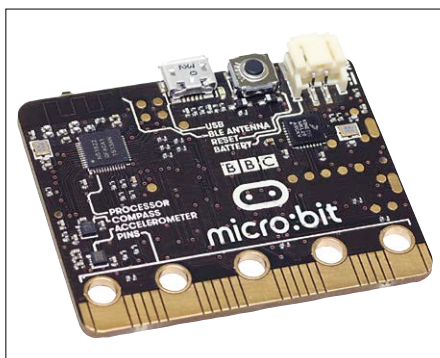
Figure 2. The BBC micro:bit can be programmed online in MicroPython.
