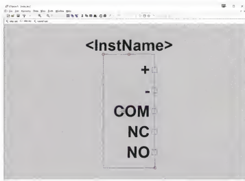
Fig.5: now we move onto creating the relay symbol by selecting Hierarchy → Open This Sheet's Symbol on the menu bar in LTspice. This is the default symbol that is created.
