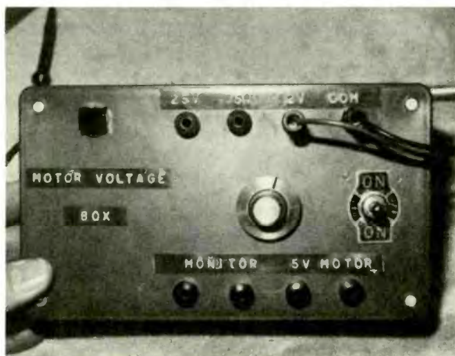
The constant voltage portion can test the various motors found in cassette, 8-track, and auto cassette players, while the 0–5 voltage source can check motors in portable cassettes, CD players, camcorders, and the like.
