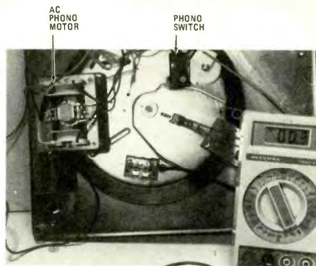
The AC phono motor may be checked for continuity with the low-ohm scale of the ohmmeter. The resistance measurement may be quite low so be sure to set the scale to low.
