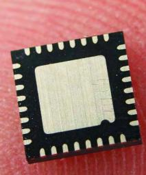
taken up by the pins compared to larger chips. The difference in area can be as much as a factor of two. Just like our example with the map, a lot of area is 'lost' by the use of connecting pins along the edge.
