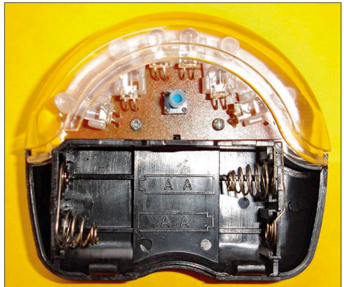
Fig. 4. The rescued rear light just waiting for a new set of batteries. Rechargeables will be a better option.
