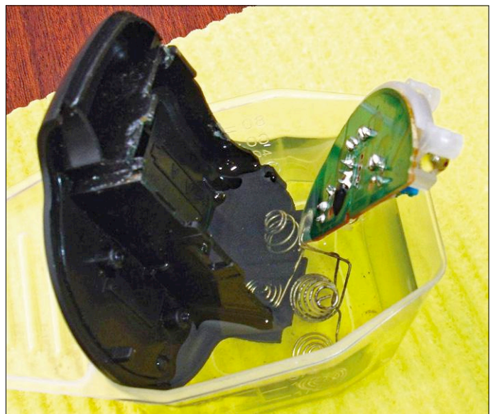
Fig. 2. The battery contacts and affected PCB area are soaked in the bath containing dish washer detergent.
