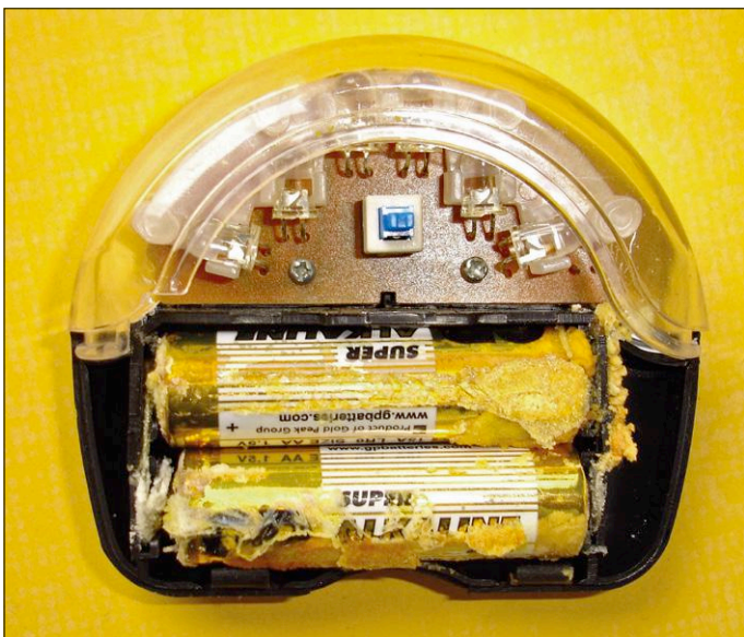
Fig. 1. After two years of neglect the alkaline batteries in this cycle rear light are exhausted and leaking.
