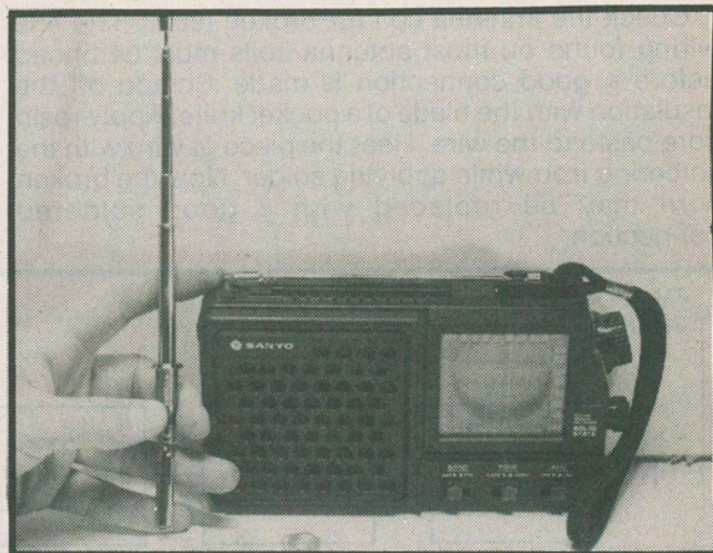
Figure 12. A universal FM dipole antenna may be installed when the original is not available. Enlarge the plastic hole with the point of a soldering iron.
