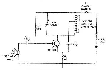
amplitude by the amplified audio signal. This amplitude modulated RF wave can be received by a nearby AM radio receiver tuned to the frequency of the emitted RF wave. The frequency of the emitted RF wave can be changed by varying the capacitance of VCI (one section of a 2X gang).
