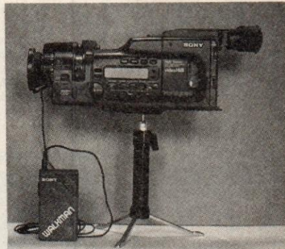
FIG. 11—THE FM RECEIVER CONNECTS to the external microphone input jack on your camcorder.
