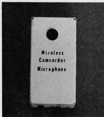
FIG. 7—A METAL CASE, like this one, provides the best possible shielding for the circuit.
