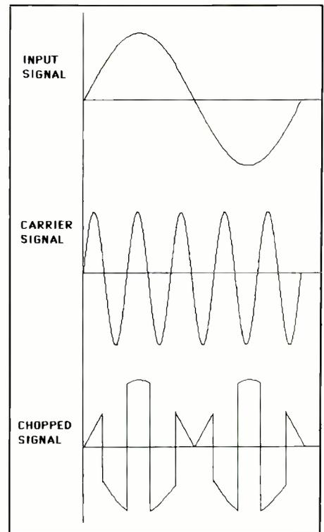
Fig. 5. How signal chopping results in amplitude modulation.
