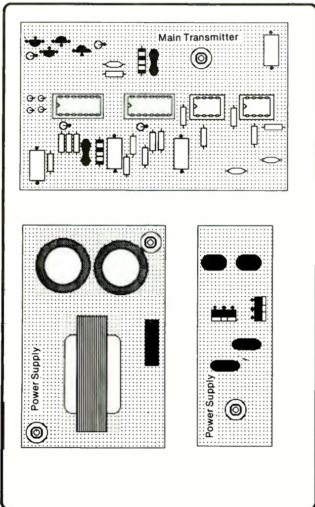
Fig. 10. Layout details for circuit-board assemblies inside enclosure. Large board at top is main transmitter circuitry. Power supply circuitry is on two smaller boards shown at bottom.
