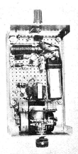
Wire the circuit board completely before mounting it in the cabinet. Keep the leads in the RF section (C2, C3, C4, C6, L1, R2, Q2) of the circuit as short and direct as possible. To prevent D1, Q1 and Q2 from being damaged, hold the leads with a pair of pliers when soldering in place.
