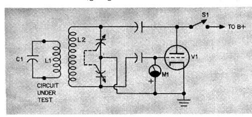
Grid-dip oscillators come in a wide variety of shapes and sixes, but all have two things in common—a tube or transistor connected as an oscillator, and a microaumeter to indicate grid or base current, Simplified vacuumtube version shown here is basically a Colpitts oscillator.
