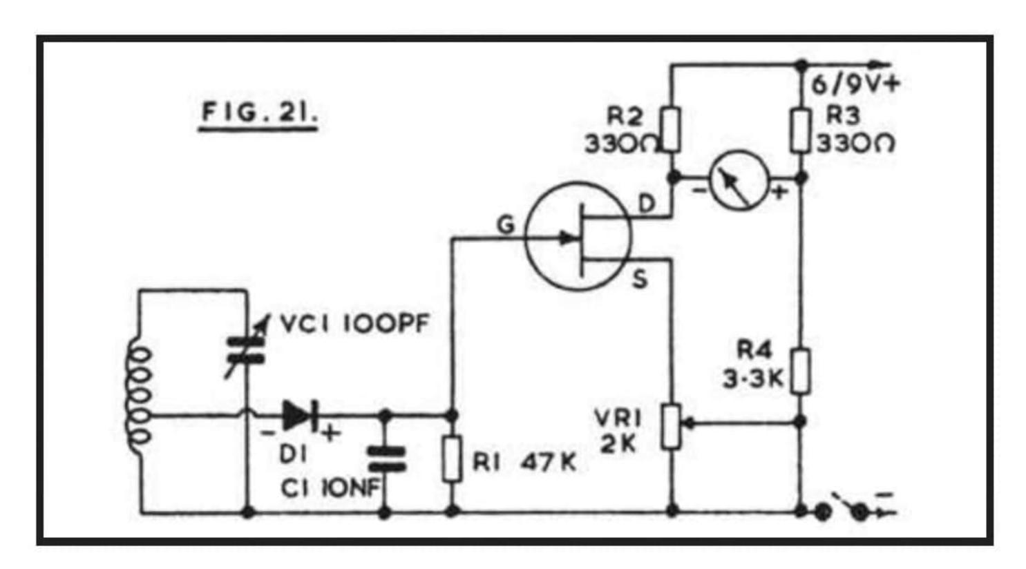
tion, VC1 tunes the inductor to resonance so that D1 produces a positive voltage across R1, for the FET gate. The meter itself is in a bridge circuit, VR1, the FET and R2 being one side, and R3/R4 the other side. Balance, or zero current through the meter, is obtained by setting VR1. Balance is then upset when the gate moves positive, and the indication can be half scale or more, so that good sensitivity is obtained.
