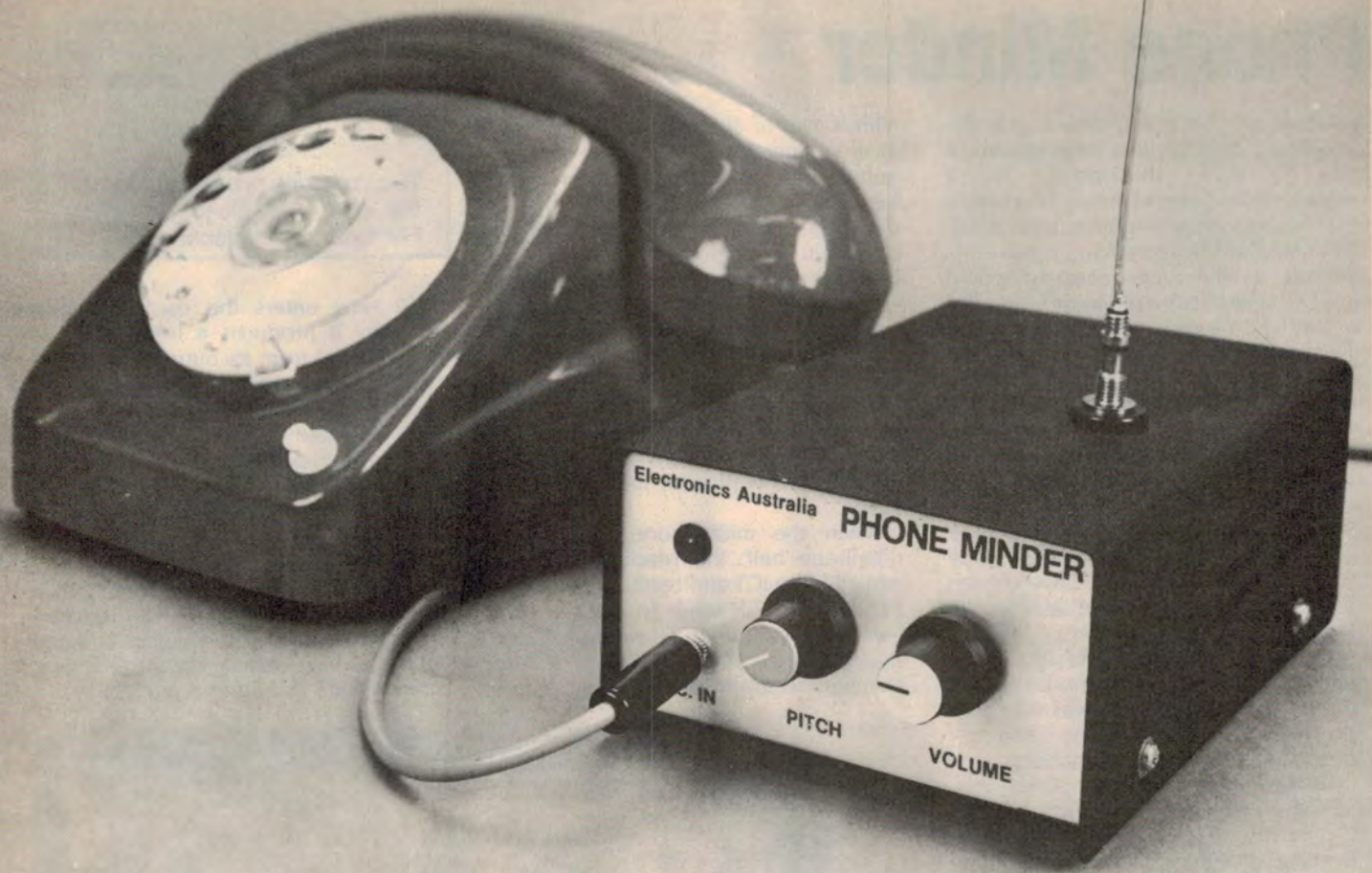
Phone Minder sits next to the telephone and uses a microphone to monitor the bell.
