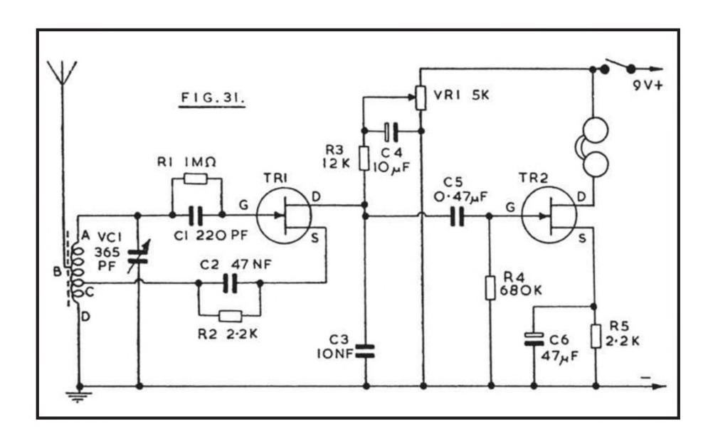
audio amplifier, operating the headphones. A complete headset is preferable for general listening, and phones of about 500 ohms DC resistance, or about 2k impedance, will give very good results here. If a miniature earpiece is wanted, this should be a medium or high impedance magnetic unit. A crystal earpiece will require resistance capacity coupling, Figure 32.
