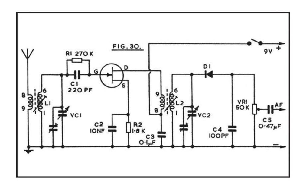
much higher level, than that from a pick-up or microphone. It may thus be convenient to retain VR1 so that output can easily be set at a suitable level.
