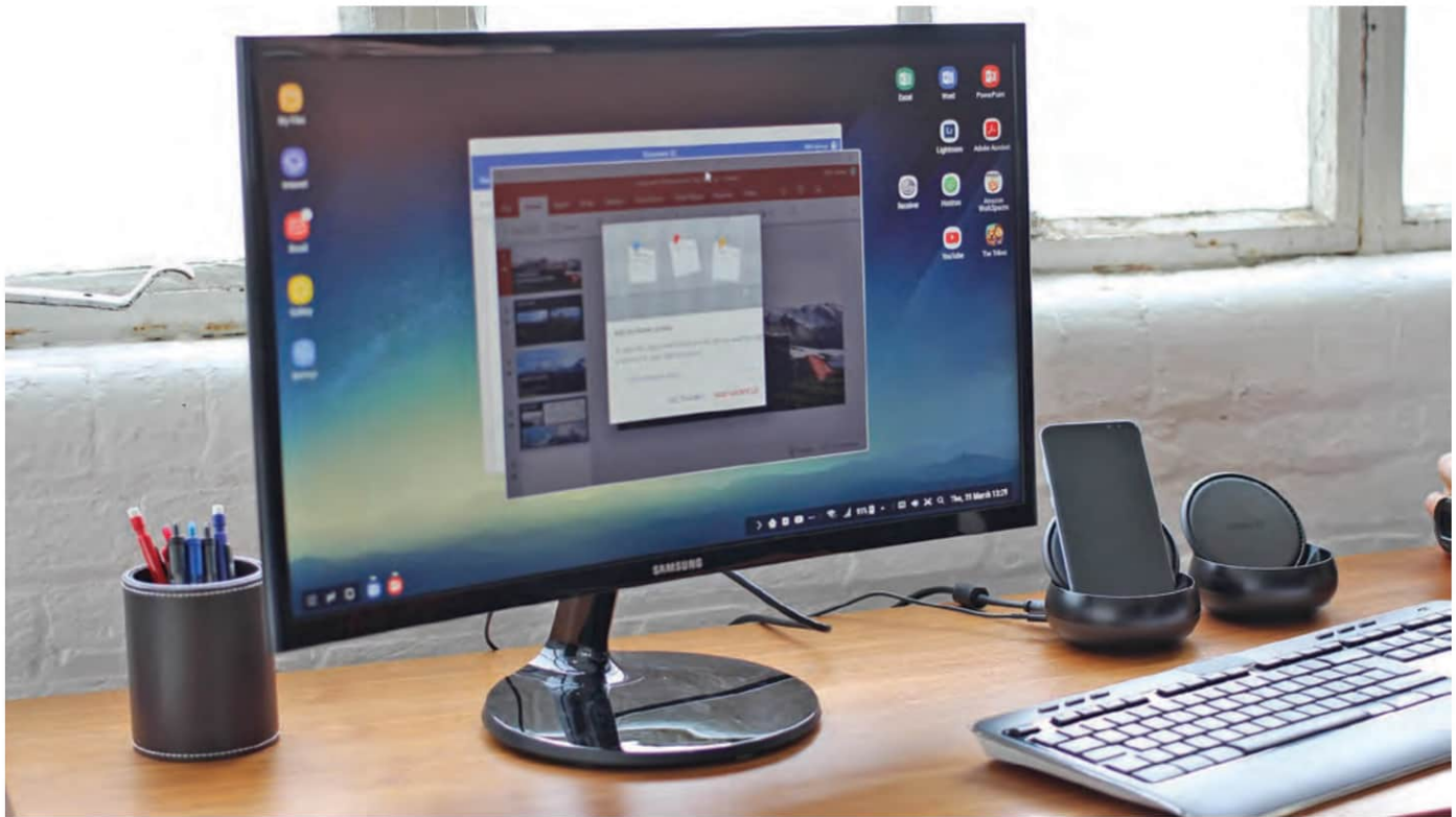
Samsung DeX with phone plugged into docking station allowing keyboard, monitor, ethernet, USB ports and mouse functions to provide desktop-like functionality. This illustrates the flexibility of the Android OS.
