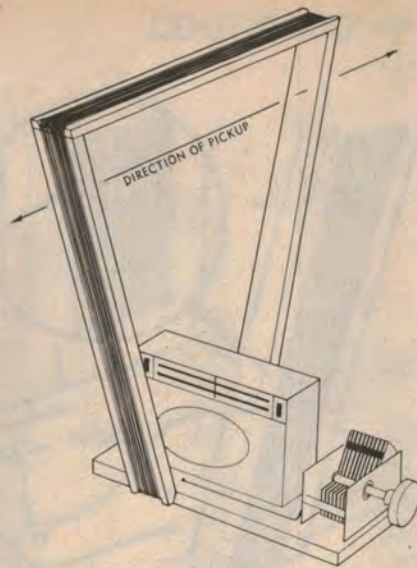
A frame aerial has obvious directional qualities. To get an accurate bearing on a distant transmitter, the frame aerial needs to be in the open, away from house wiring, metal roofing, etc.
