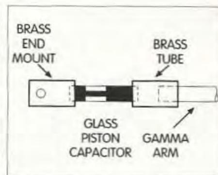
**Fig. 3.** The first attempt at constructing the gamma match section with a glass piston capacitor soldered to small sections of brass tubing for connections to the mounting insulator and gamma aluminum rod.
