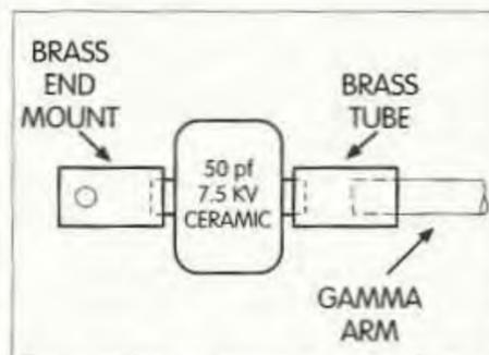
**Fig. 4.** Final gamma match capacitor construction using a 50 pF ceramic high voltage capacitor attached to brass tubing. Near end swaged for nut and bolt attachment and the other end inserted into the original aluminum gamma match arm. Attached with a 4-40 bolt through both brass and aluminum rod.
