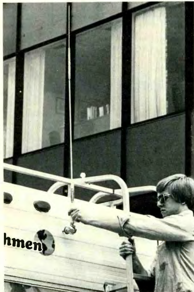
Fig. 6—A few mobile antennas such as this Breaker Corp. Model 10-500 are specially designed for use on fiberglass-bodied RV's, campers and sports cars.
