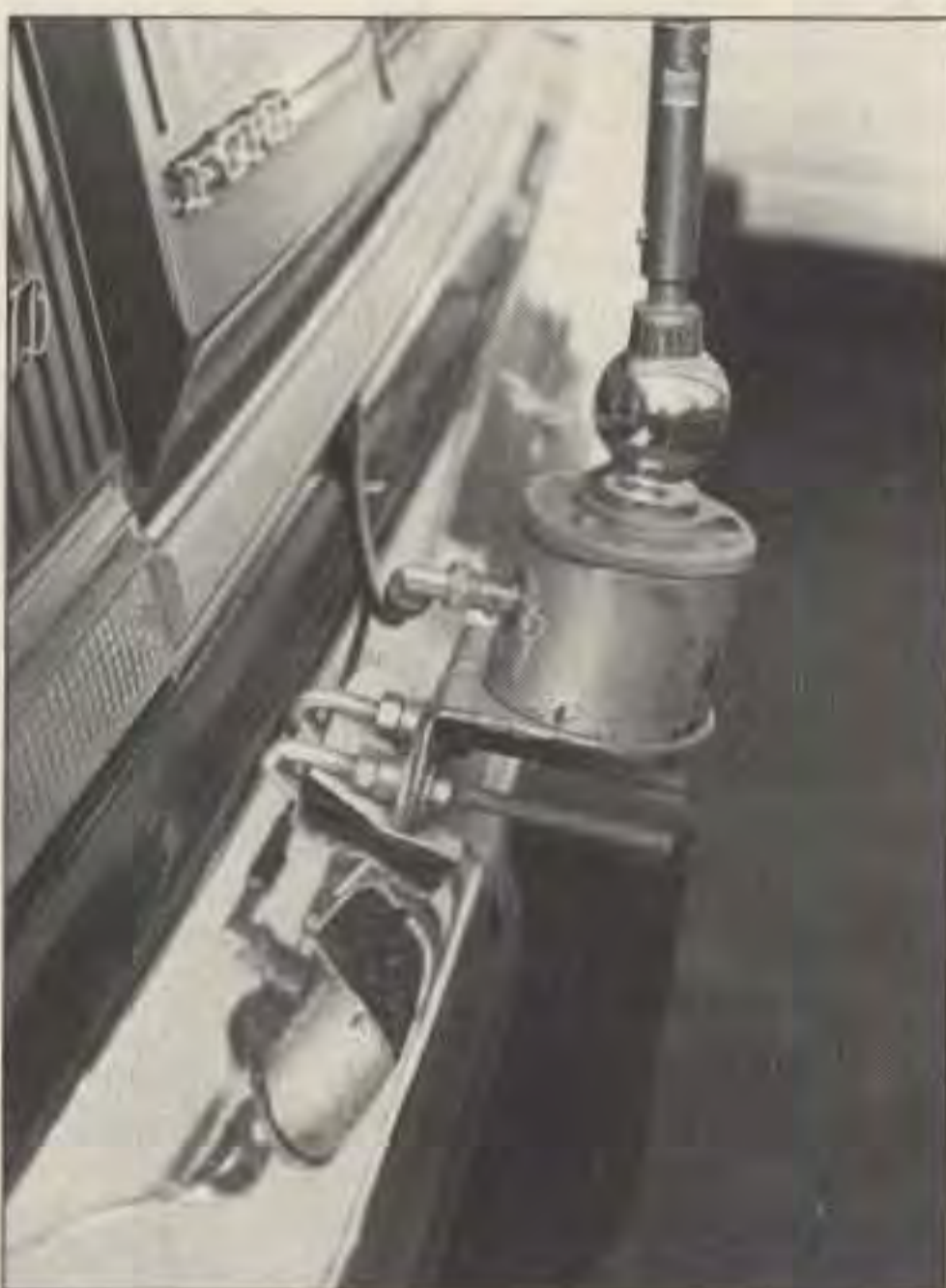
A BNC connector for the enclosure makes it easy to attach coax to the mount.
