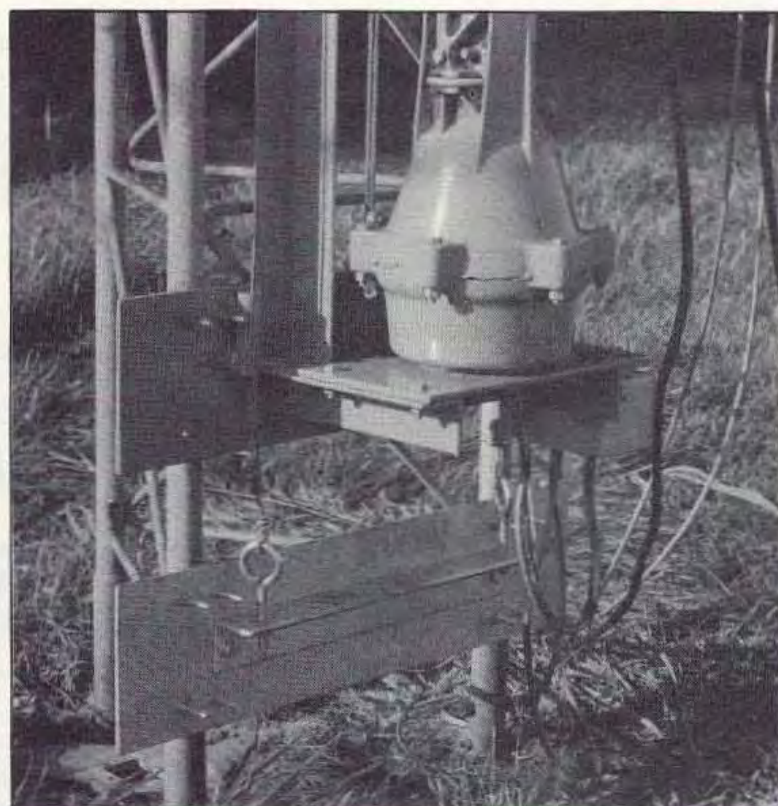
Photo B. The rotator and guide wires attached to their eye bolts and passing through the guides on the elevator.
