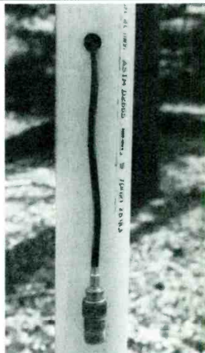
FIG. 5—EXITING coaxial cable and connector appear at bottom of the mast.
