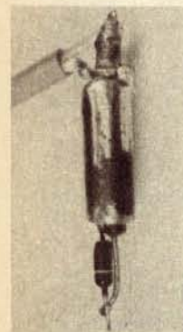
A photograph and diagram showing the construction of the slotted line probe assembly.
