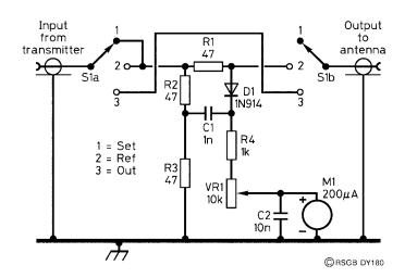
Figure 1 Resistive SWR meter, circuit diagram
