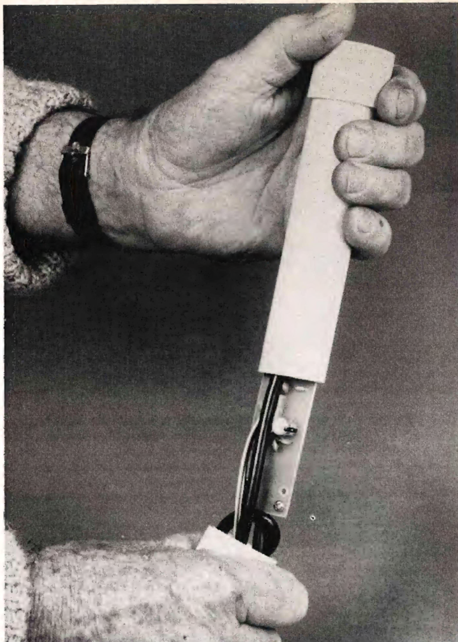
The PCB has been specially designed to slide into a 32 x 150mm length of plastic conduit which is then fitted with end caps for weatherproofing. The input, output and power supply leads are fed through holes drilled in the bottom end cap and secured to the mast using cable ties.
