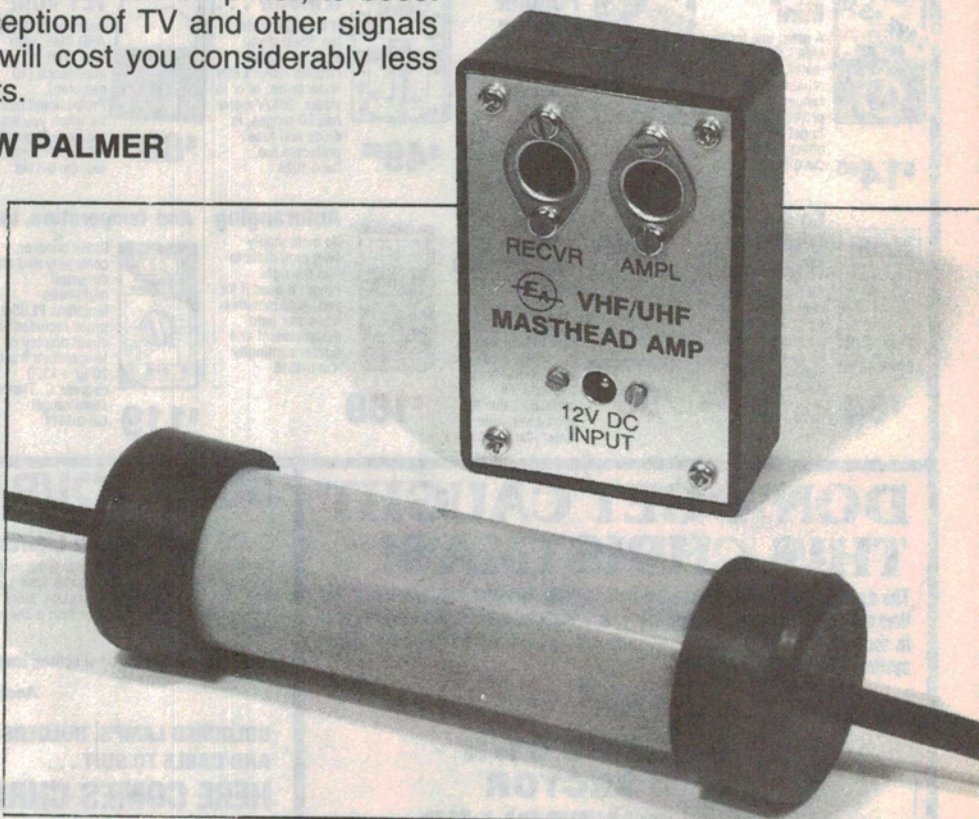
The complete project consists of two parts: the amplifier itself, in the PVC tube in the foreground, and the power feed unit.
