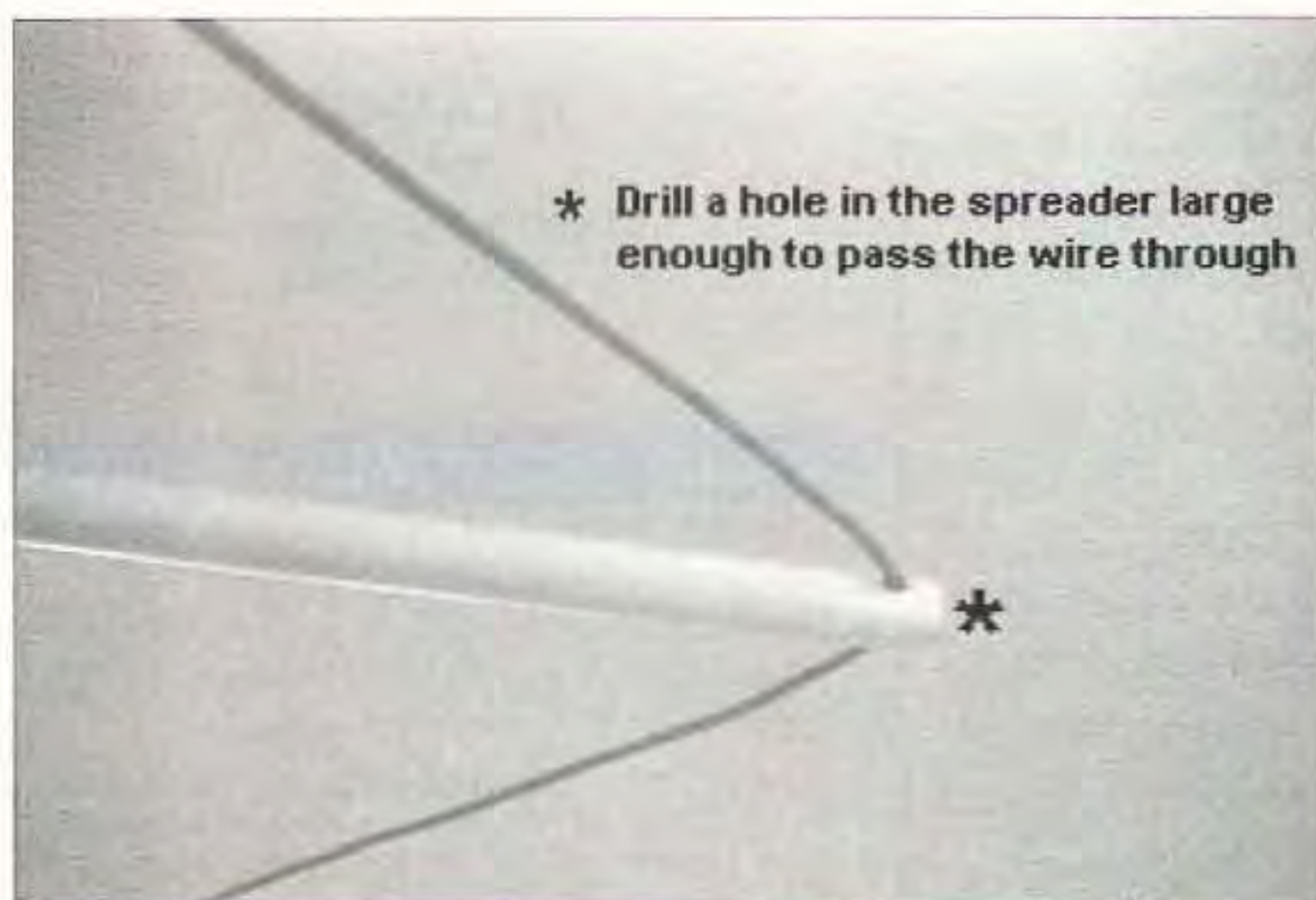
Photo G. Construction of the non-fed corner of the loop.
