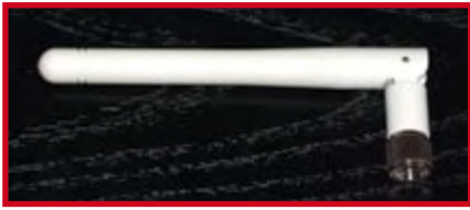
Figure 3. Quarter-wavelength stub antenna suitable for a WLAN router or access point.
