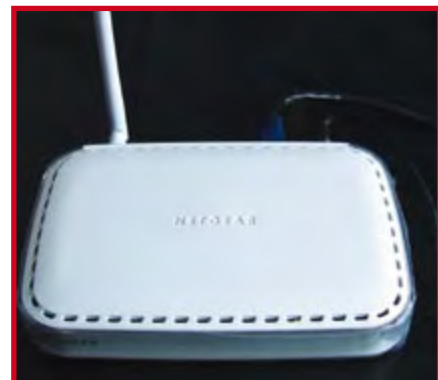
Figure 2. A typical access point: sometimes these are used to help reduce the length of antenna cable needed.
