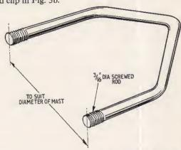
Fig. 5a. This 'U'-shaped cleat is fixed to the upper holes in the bracket (see below) to hold this bracket firmly to a vertical hole
