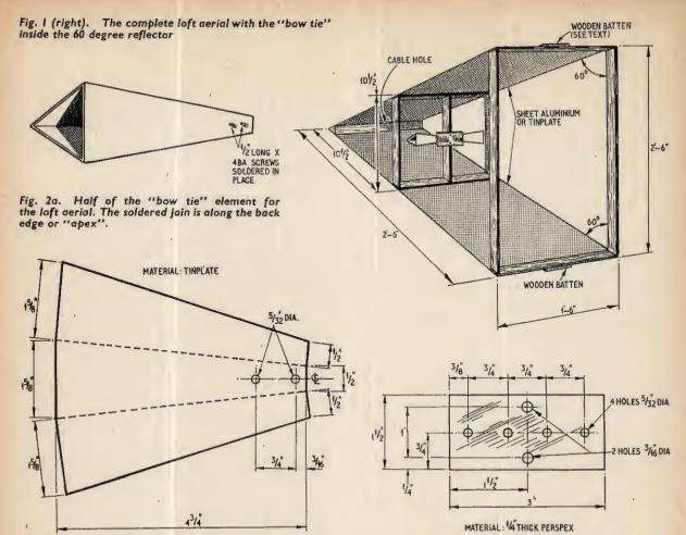
Fig. 2b. Constructional details of the "bow tie". Two are required to be made from sheet timplate
