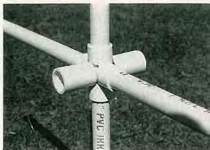
FIG. 4—A CLOSEUP VIEW OF THE COUPLING assembly used on the driver and second director elements. Note that the reflector and first director elements have only one coupling cemented to the cross-tee.
