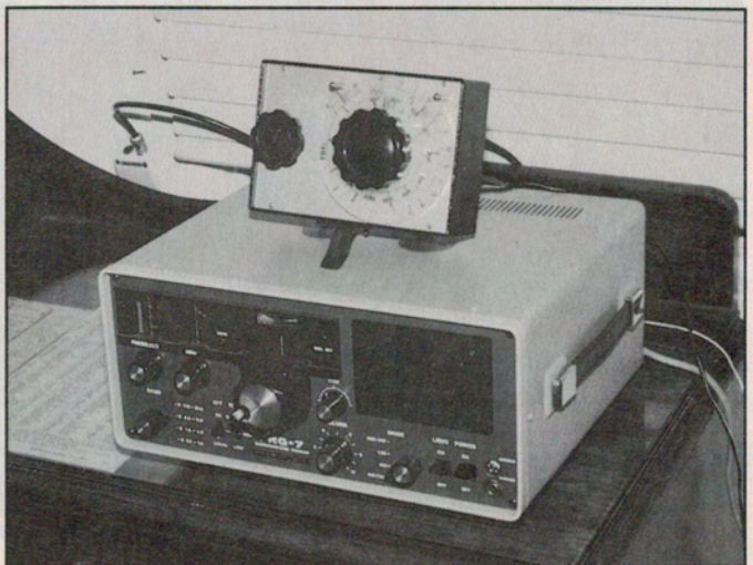
This photo shows the antenna control box in position on top of the receiver and connected with coax cable to the wall socket.
