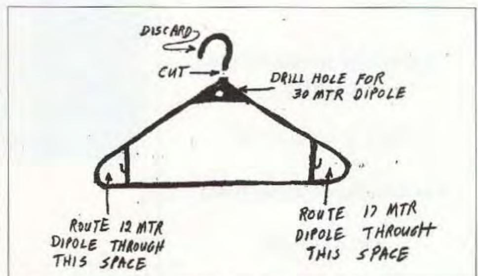
Fig. 2. Preparation details for clothes hangers.
