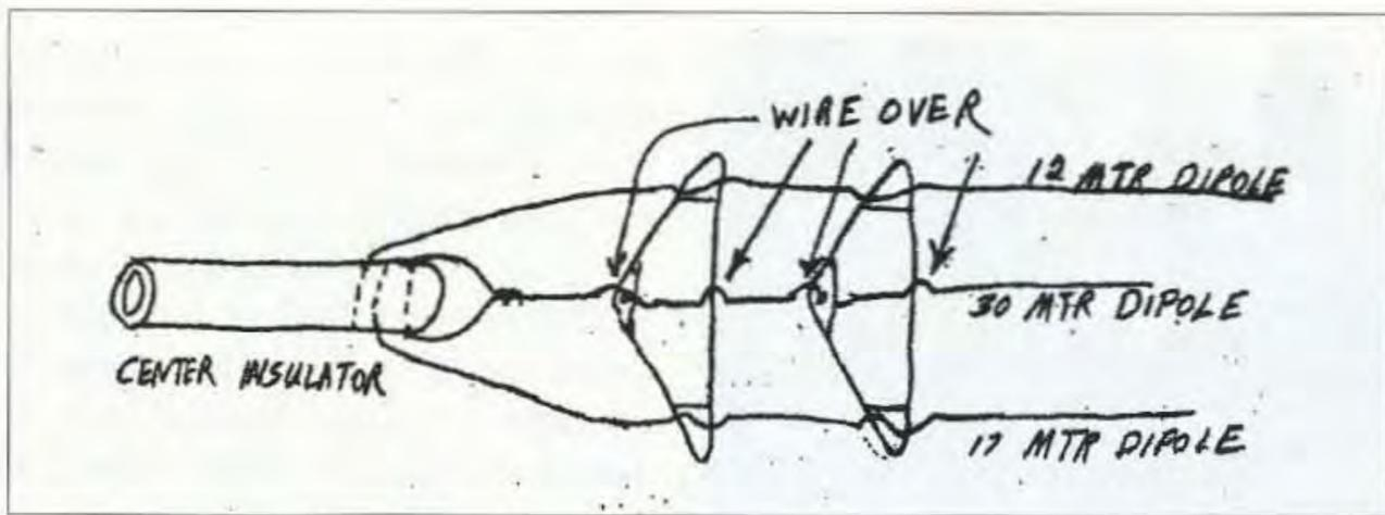
Fig. 3. Wiring detail for clothes hangers.
