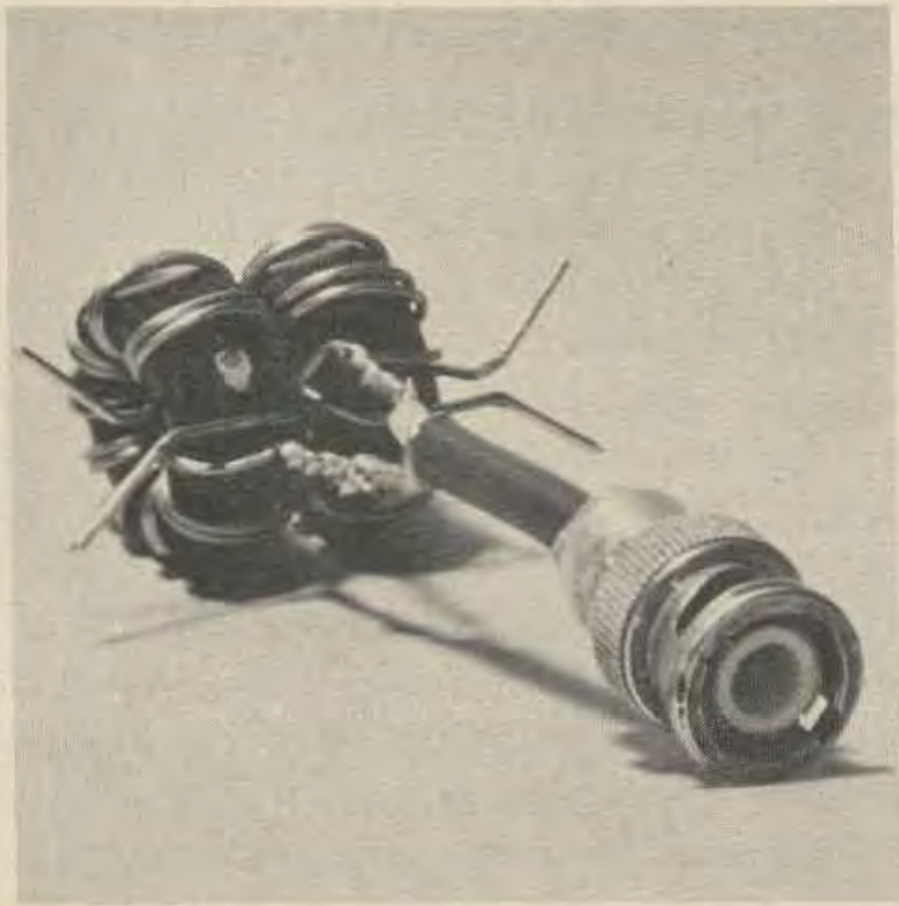
Fig. 3. This shows the quadrature coils before encapsulation. Two No. 57-1736 Permacor cores are wound with No. 16 Beldsol wire, in a bifilar fashion. This pair is for 6 meter sample, sent to Wayne Green for testing on that band.
