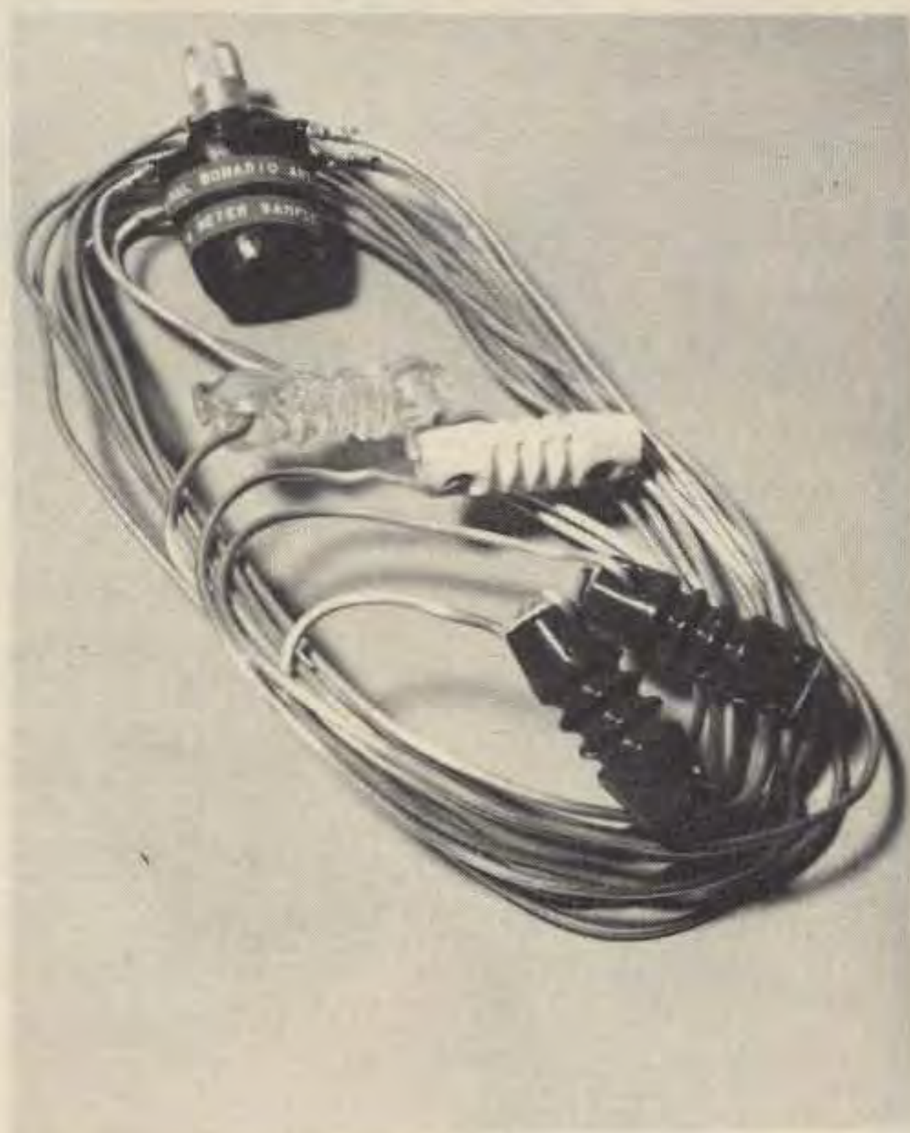
Fig. 5. The TQA is ready to be shipped. The entire antenna and insulators are easily contained in an old shoe box. With aluminum ground wire elements, the weight was very little.
