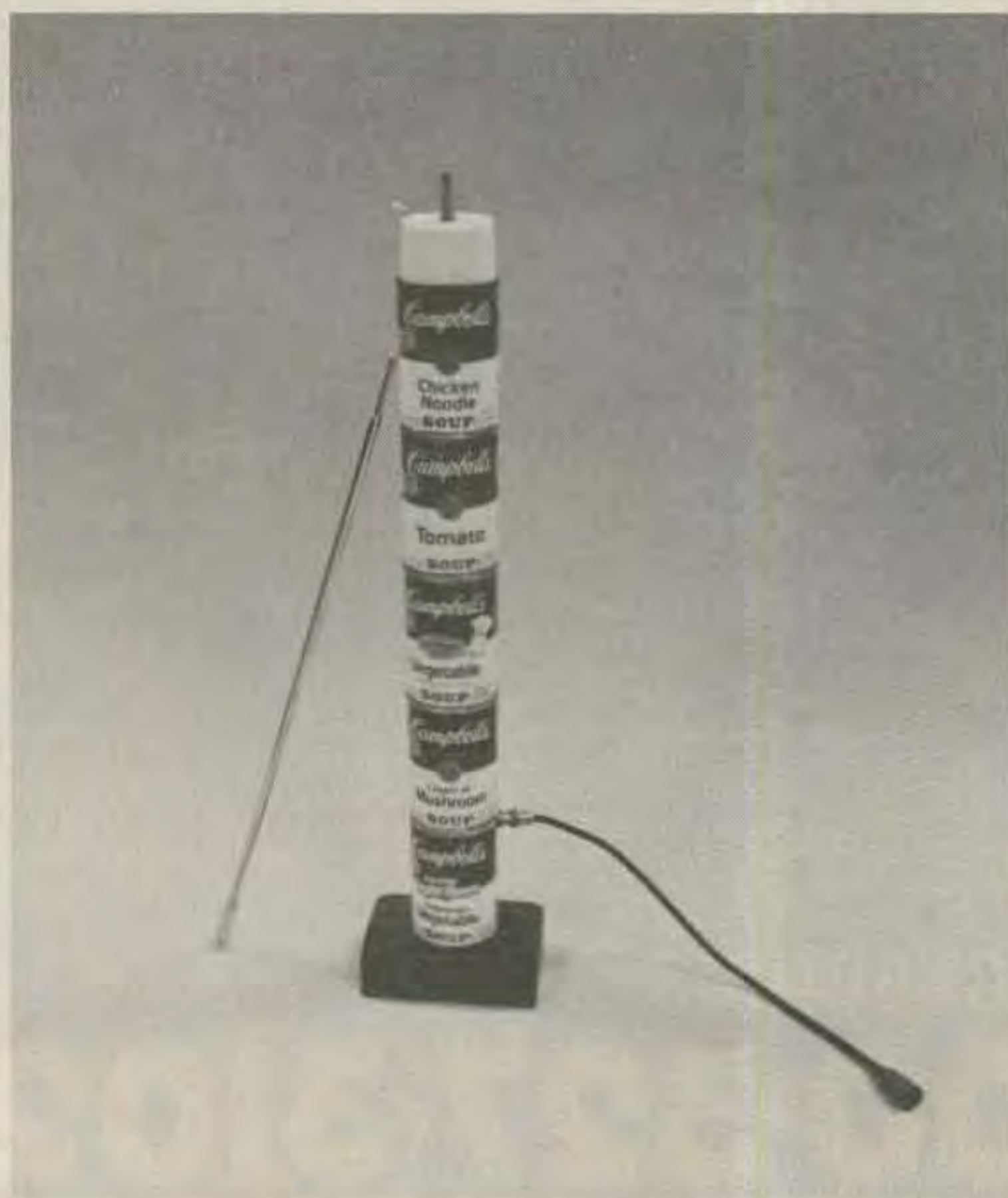
Two-meter soup can antenna.
