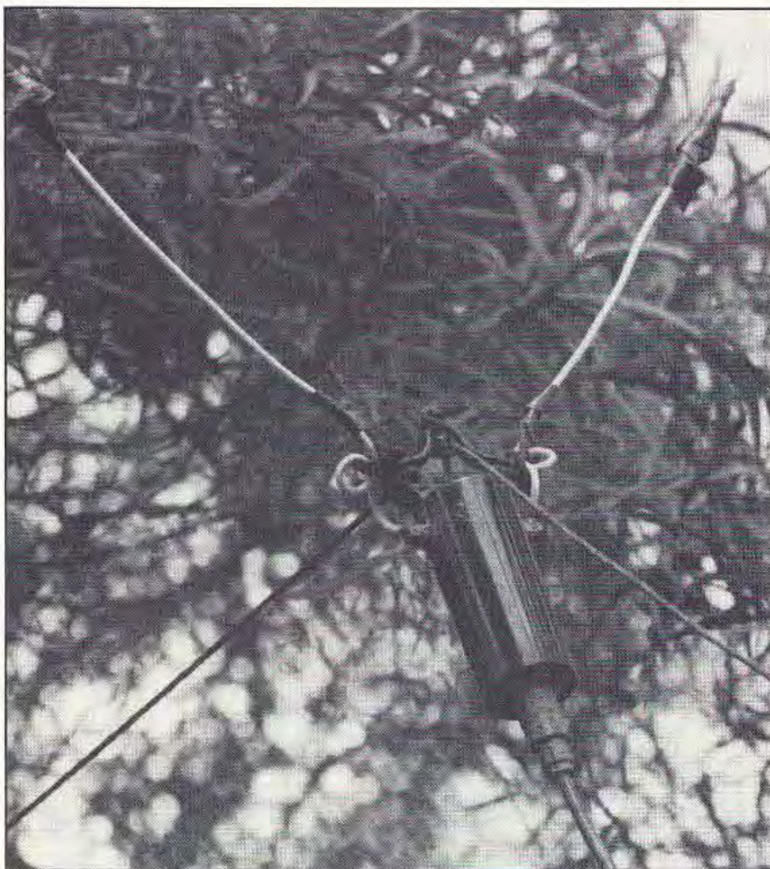
Photo A. The Hula Loop driven element at its feed point. Note the 1:1 balun.
