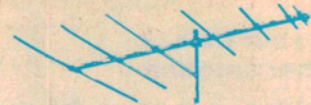
Figure 5. A typical log-periodic beam antenna (horizontally polarised here). All the elements are split in the centre and 'cross-connected' to the next in line.
