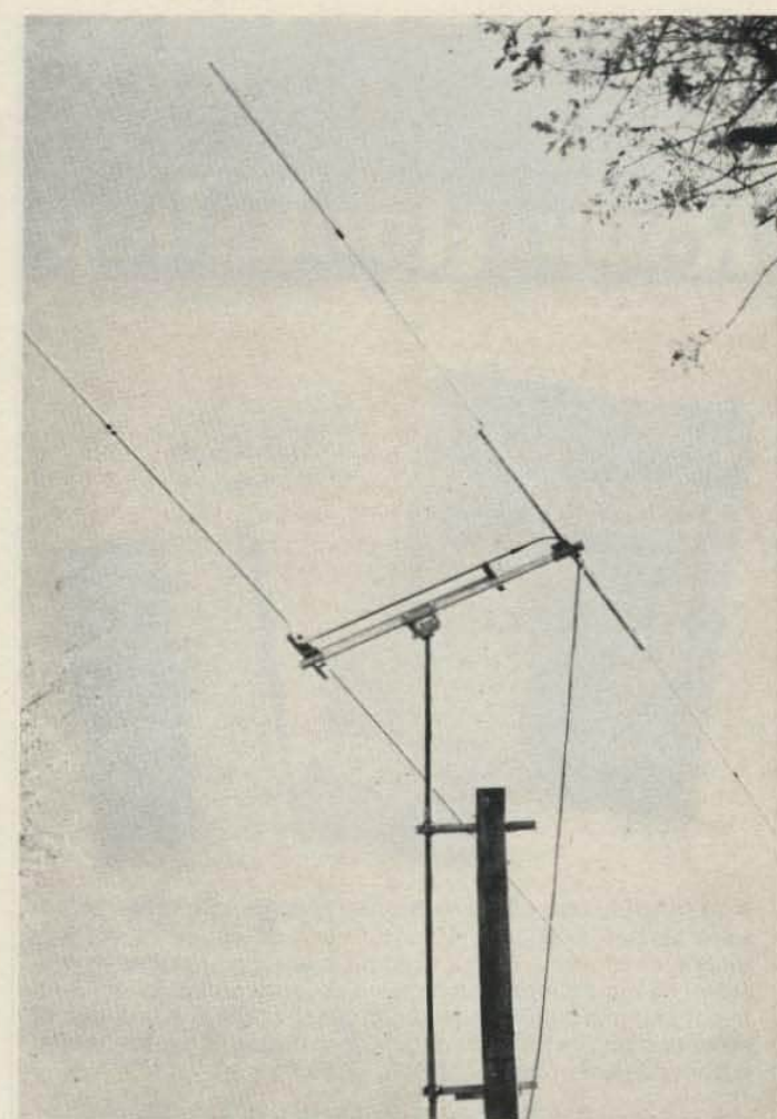
Fig. 6. LB-2 15-meter array. The split driven element is at the left in this photo. The director element, right, is insulated from the boom but grounded to it at the exact center to reduce noise pickup. Note coax line connection at end of 53-inch tube. As shown, maximum radiation will be toward the right. Maximum gain (over a half-wave dipole) is 5.3 dB. The rotator (not shown) is an AR-22 heavy-duty TV type.
