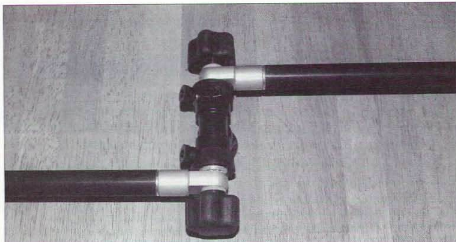
Photo B. Center insulator and position adjustment knobs for the Buddipole.
