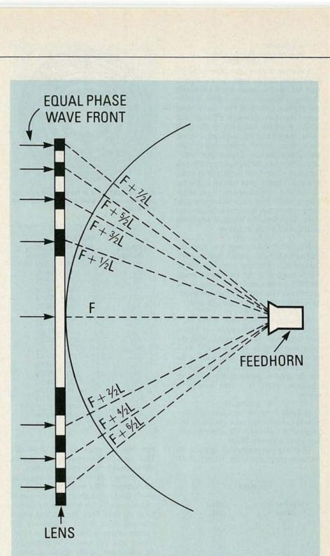
FIG. 2—DESTRUCTIVE INTERFERENCE. Waves arriving at the focal point inside the feedhorn from alternate ½-wavelength zones interfere destructively.
