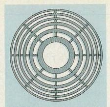
FIG. 3-FRONT VIEW of the plywood lens. The non-cross-hatched areas would be cut out of an actual lens.
