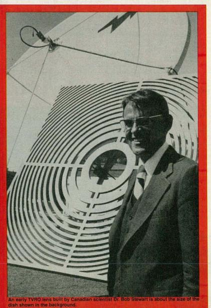
cause the design comes from the study of optics, not communications. In fact, there has been so little published research concerning the use of Fresnel lenses for satellite reception that the field must definitely be considered experimental. Although there are a few isolated examples of the Fresnel lens in actual use for satellite reception in Canada (British Columbia), commercial production of such lenses appears to be nonexistent.
