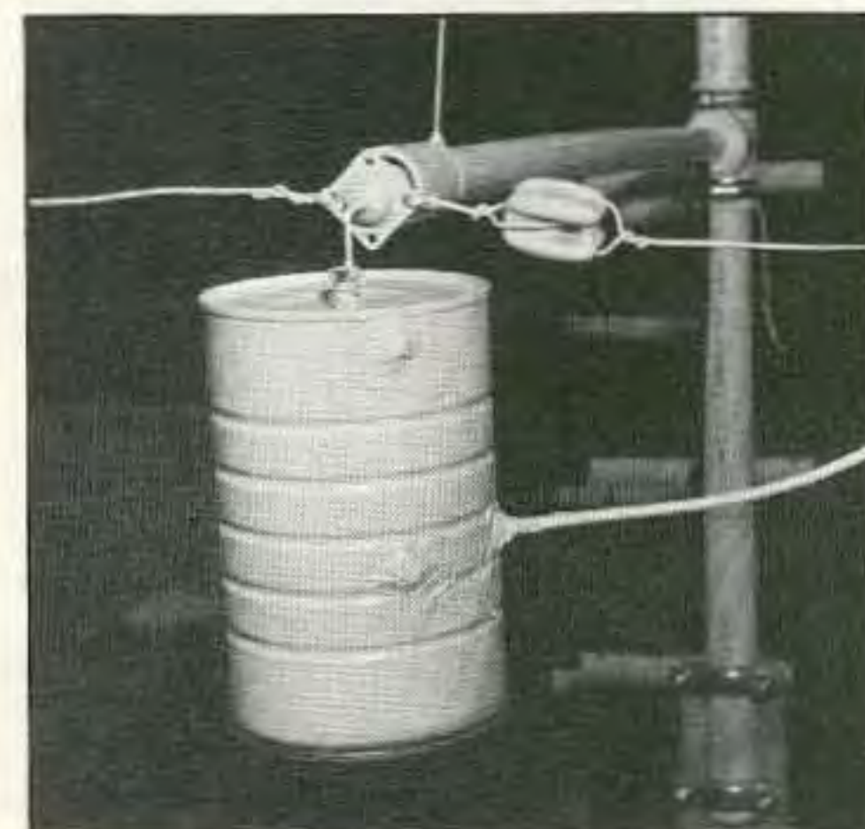
Photo F. The coffee can feedpoint is supported by a 1/2-inch PVC pipe through which passes the 50 ohm coax feedline. Note how the SO-239 chassis connector is rigged. One end of the driven loop is soldered to the left corner of the connector base. The other end of the loop is supported by, but insulated from, the opposite corner of the connector base. A wire bolted to the can is soldered to the center contact of the connector. The holes in the can have been sealed with silicon sealer, and the outside painted to prevent rust.
