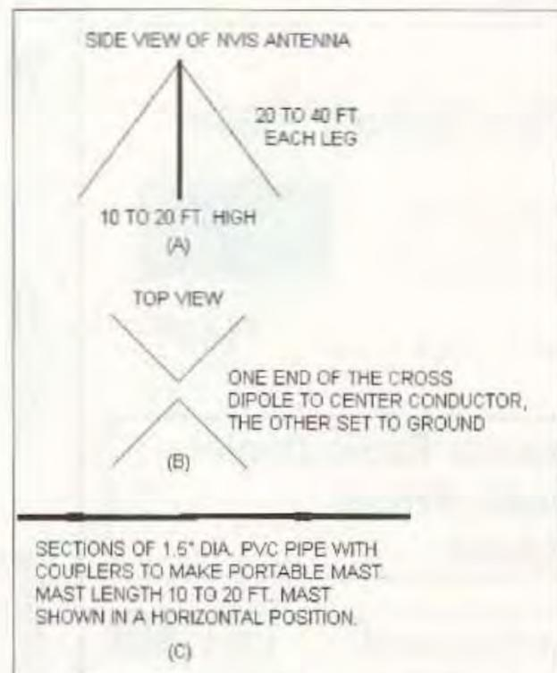
**Fig. 1.** NVIS antenna details.
