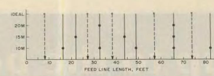
Fig. 5. Feedline resonant lengths are shown by dots and solid lines; these lengths should be avoided. Ideal lengths for a 20-, 15-, and 10-meter feedline are shown by an X with a dotted line. Resonant frequencies chosen for this chart are 14.175, 21.225, and 28.500 MHz, representing an approximate median for each band.
