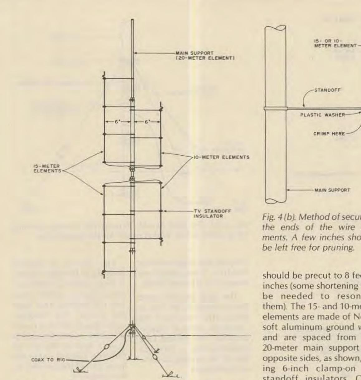
length will depend, to some extent, on how close the antenna is to trees and other obstructions. (The antenna should be located so that it cannot fall on utility lines!)
